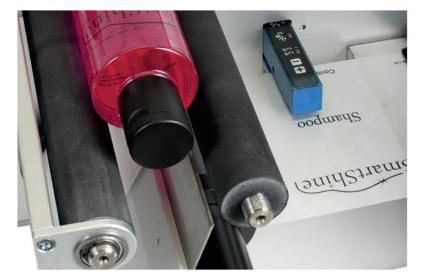
The labels are read by a fork photocell that read the transparency difference between labels and liner. It is also available an ultrasonic sensor which read the thickness difference between labels and liner in the case of transparent labels.
