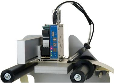
DWR ROUND can be equipped with a inkjet coder with HP technology for writing variables data such as date time in real time, bar codes, texts with a maximum height of 12.7 mm at 300 dpi resolution and speed synchronized to the feeding label.
